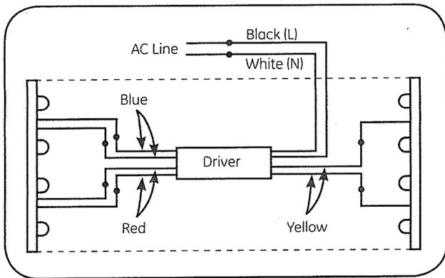
**4C Four Tube Fixture:** Connect the black (L) and white (N) wires of driver to black and white wires of AC line, respectively. Connect the blue wire of the driver to one set of lampholders at one end. At the same end connect the red wires to other set of lampholders. At the opposite end, connect yellow wires to lampholders.
